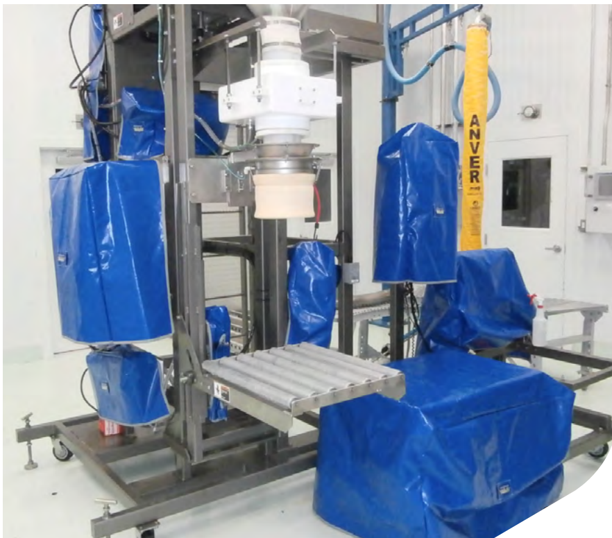
Shannon Rain Shield in use at Pharmaceutical Manufacturing Facility
