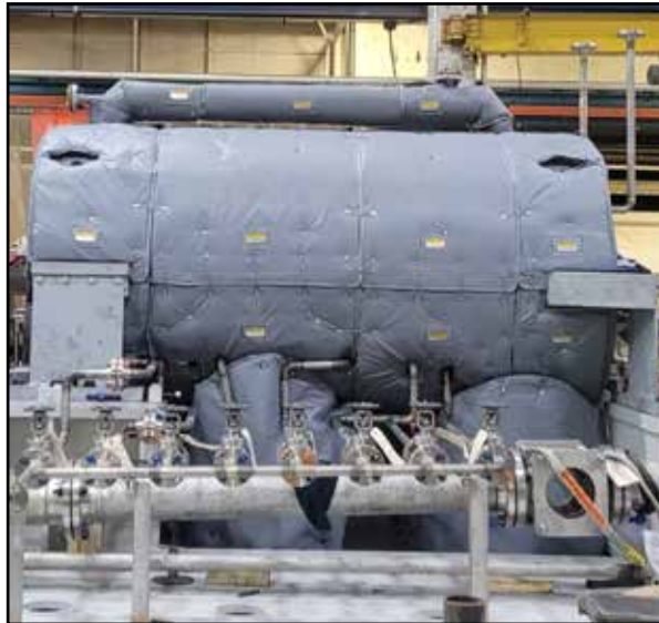
LT450A-TT COMPRESSOR HOUSING (8 dBA REDUCTION)
