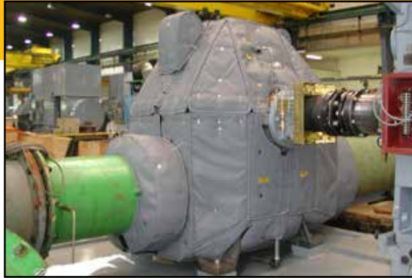
LT450A-TT SPLIT CASE PUMP 24x20-36 (6 dBA REDUCTION)
