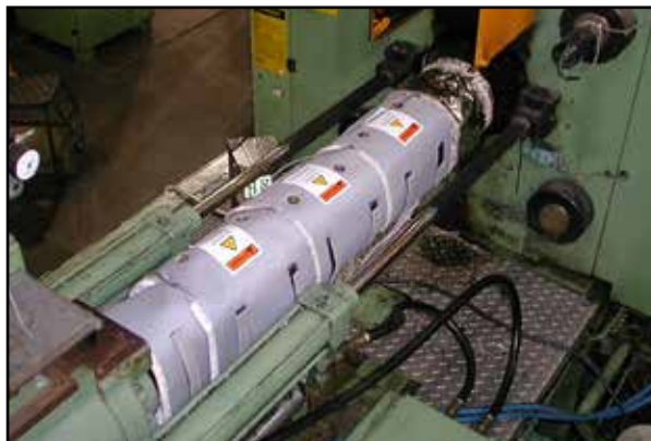
LT550SG - D-RING STRAP, VECRO TAB EXTRUDER BARREL
