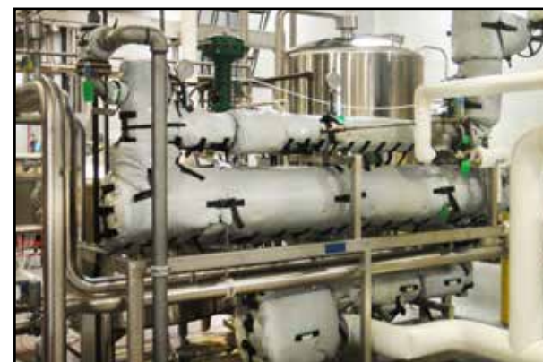
LT550LFP - SIDE RELEASE BUCKLE STEAM PASTEURIZER
