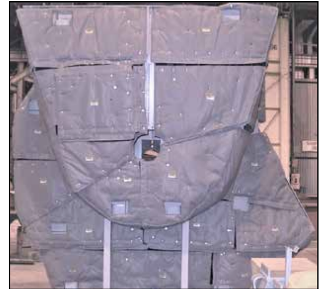
LT450A-TT INDUSTRIAL FAN HOUSING (8-10 dBA REDUCTION)
